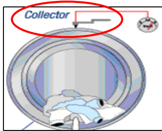
Brush contactor degrades over time
