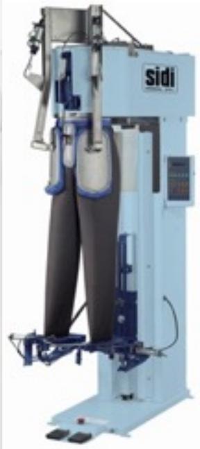
Universal Pneumatic topper with pneumatic tensioners and special paddles for pleats pressing . Steam heated waist form . Possibility of steaming and blowing before locking of the pneumatic paddles.
