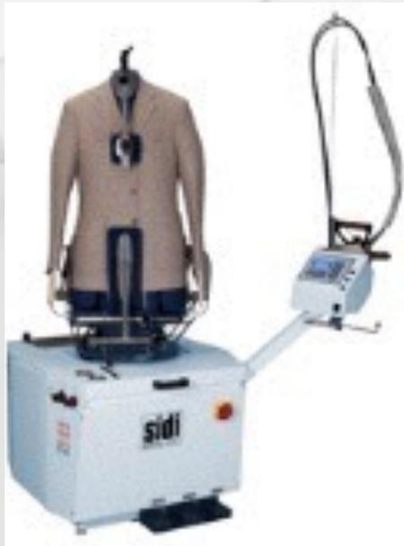
Tensioning form finisher, designed to fulfill demands of a Wet Cleaning pressing system that requires vertical tensioning for perfect seam finishing and fabric "revitalising". It features a special tensioning system for the garment being processed and the powerful hot air flow provides a high class finish. Automatic positioning of the dummy is accomplished using a photocell.
